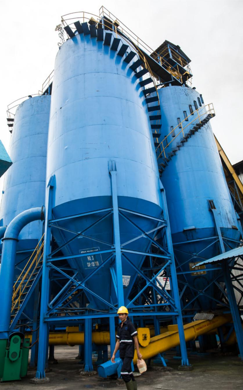
Silos for bulk storage of palm kernels
